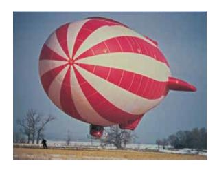
elevators are the co-pilot's responsibility. The single rudder is located on the bottom fin to take advantage of propeller wash. Thus, by increasing airspeed, the response to rudder deflection is increased. Turning rates have been checked on several occasions and result in 3° per second at half power and 4° per second at 75 % power (approx. 15 knots). Both pitch and yaw control of the airship have proved to be acceptable.
